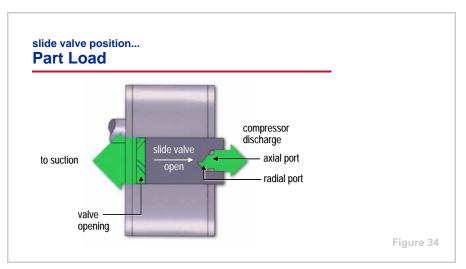
At part load, the slide valve modulates toward the open position. The opening created by the valve movement allows refrigerant vapor to bypass from the rotor pockets back to the suction side of the compressor. This reduces the volume of vapor available for the compression process. It also reduces the amount of rotor length available for compression. In this manner, the volume of refrigerant that is pumped by the compressor is varied, unloading it to balance the existing chiller load.
